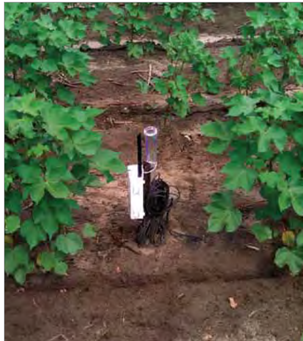
Figure 6.4 – A Decagon EM-50g data logger installed in-line with cotton plants.
