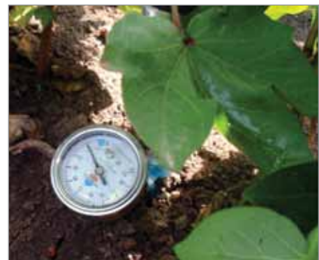
Figure 6.1 – A tensiometer installed in a cotton row.
