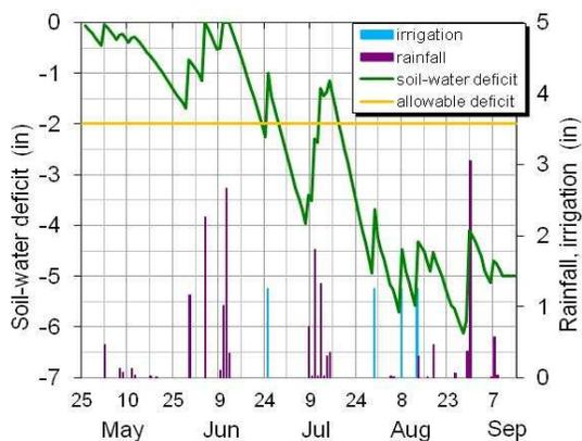
**Figure 11. Soil-water deficit estimated for 2012 using a spreadsheet water balance model.**
